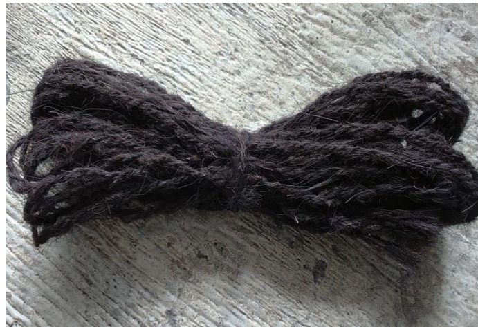
Figure 3: Sugar palm ropes (Courtesy of Mr Indra Yana, CV Sumber Mulya, Tasikmalaya, West Java)
